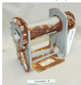
Winches exposed to acid washing and accelerated salt spray testing
