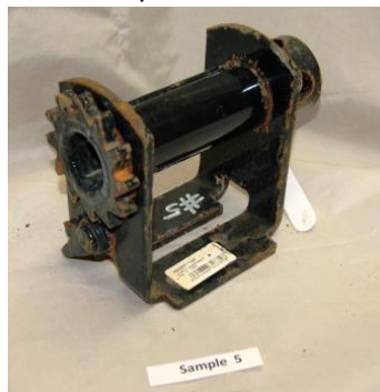
Winches exposed to acid washing and accelerated salt spray testing
